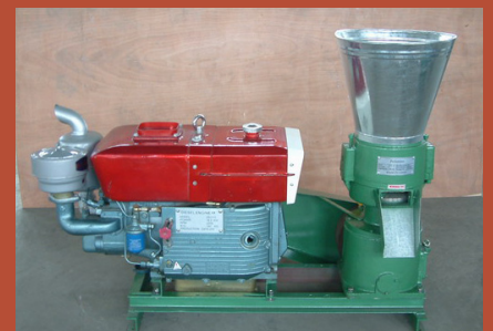
Portable pellet mills will be used on-site to convert Russian olive and saltcedar biomass into marketable biofuel pellets.
